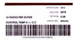
Labels printed in 'picket fence format: White lines running through the height of the bar code.
